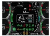
angle from the operators seat. There is no need to perform a daily calibration before beginning operation. Just set the desired slope percentage or match a pre-existing slope and begin to grade.
