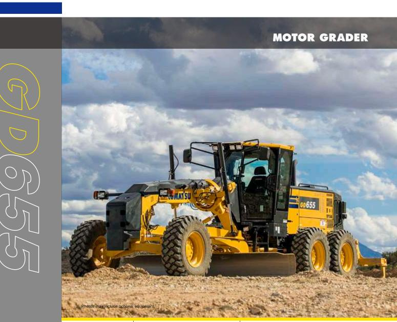
HORSEPOWER Net: 218 HP 163 kW Gross: 221 HP 165 kW **OPERATING WEIGHT** 38,250 lb 17350 kg 42,946 lb 19480 kg (with ripper) **BLADE LENGTH 14'** 4.27 m
