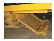
around the underguard helps prevent debris from entering.
