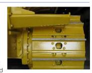
dozer. The additional 3" of clearance between the track shoes and the dozer makes clean out and maintenance procedures
