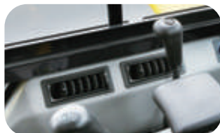
Heater with fresh air vents
