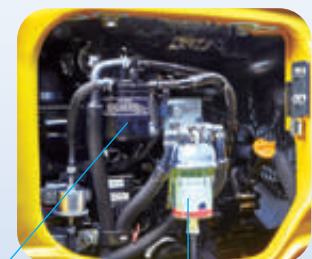
Fuel pre-filter (with water separator)
