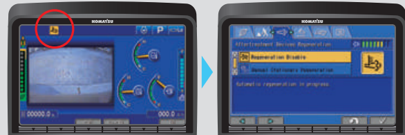
Aftertreatment device regeneration screen
