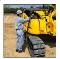
The auxiliary hydraulic circuit return filter has been relocated for easier ground-level access alongside the windshield washer tank
