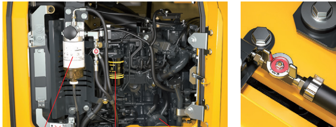
Fuel pre-filter (With water separator) High efficiency fuel filter Engine oil filter Fuel drain valve
