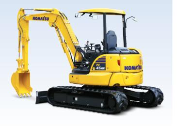
A powerful Komatsu 4D88E-7 engine provides a net output of 38 HP (28.3 kW). This engine is EPA Tier 4 Final emissions certified.
