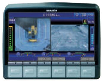
Monitor display provides individual camera views as well as a bird's eye view.
