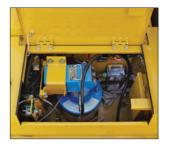
**Grease gun** located in compartment underneath the front step provides easy ground level access.
