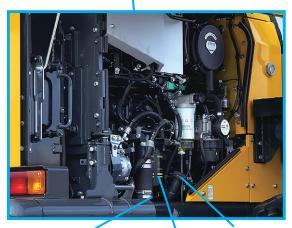
Engine oil dipstick Fuel filter Engine oil fill
