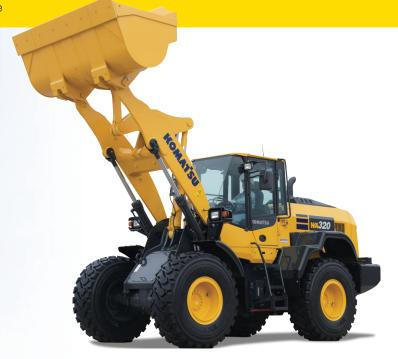
A powerful Komatsu SAA6D107E-3 engine provides a net output of 123 kW 165 HP with up to 3% improved fuel consumption. This engine is EPA Tier 4 Final emissions certified.
