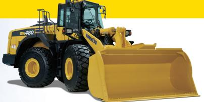
The **Yard Loader arrangement** features a 7.2 yd<sup>3</sup> genuine Komatsu high performance bucket, low profile 775/65/ R29 tires, an improved brake cooling system and a heavier Yard Loader counter weight, and is designed to three pass typical on-highway trucks.
