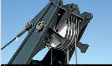
Four polymer head sheaves with maintenance free sealed bearings
