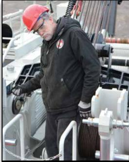
Counterweight removal controls located on work platform at the rear of the crane
