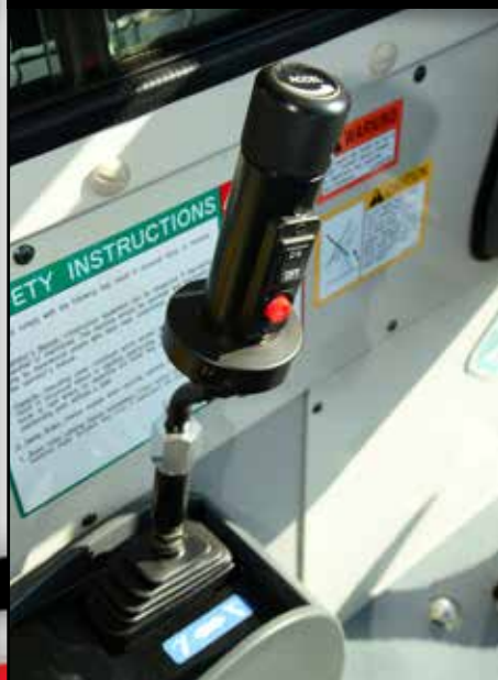
Variable hand throttle for infinite main pump control.
