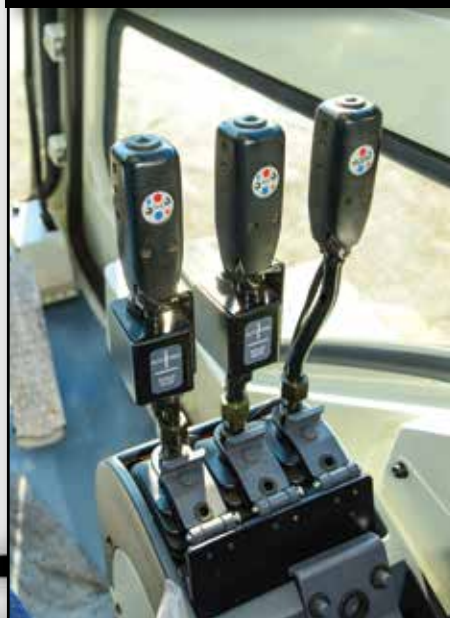
Pilot-operated armchair controls with adjustable sliding console
