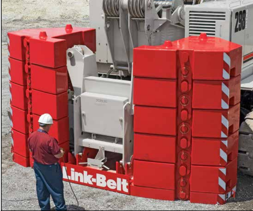
Counterweights lower completely to the ground
