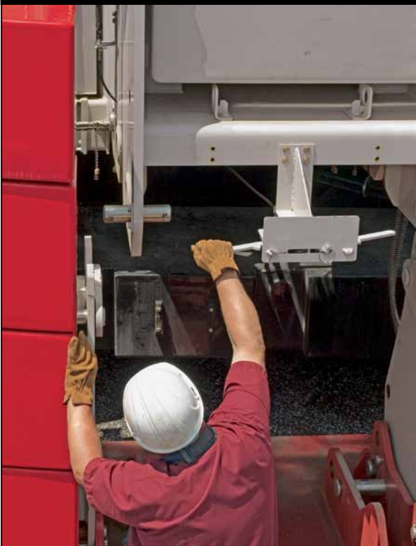
Unlatch cylinders and tray from counterweight then retract cylinders for transport
