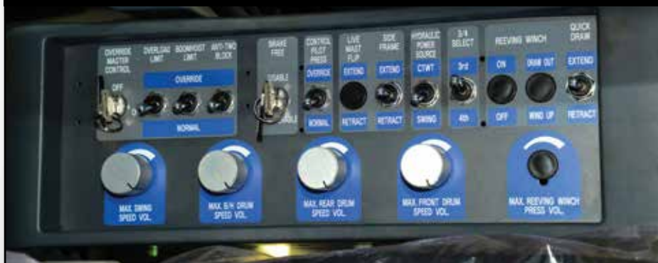
Hydraulic flow volume for precise control
