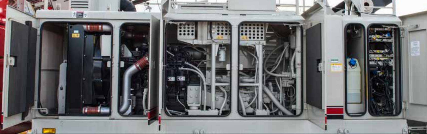
Excellent access for all routine engine and hydraulic maintenance
