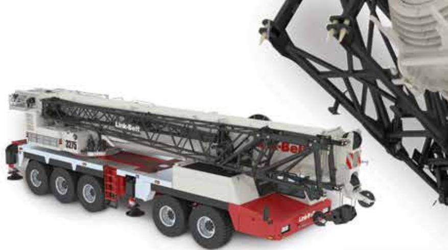
12-40-67 ft | 3.6-12.2-20.4 kg three-piece bi-fold lattice attachment with 2°, 15°, 30° and 45° manual offsets and 2°-45° hydraulic offsets
