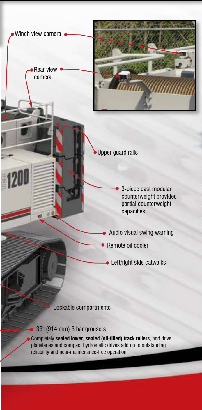
Excellent access for all routine engine and hydraulic maintenance
