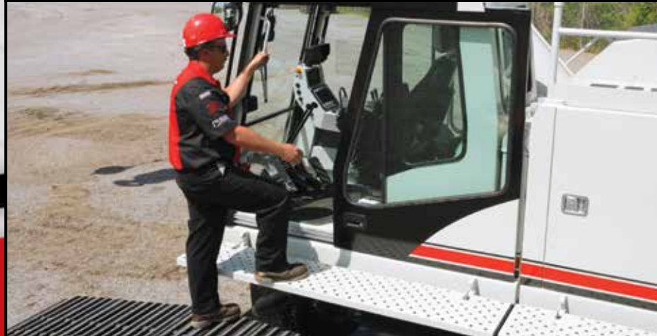
Non-slip safety strips, extended length catwalks, sideframe steps and upper guard rails provide sure-footed access to the crane upper.
