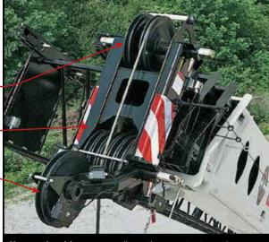
**Hammerhead boom** nose allows the operator to work at high boom angles without fouling wire rope.
