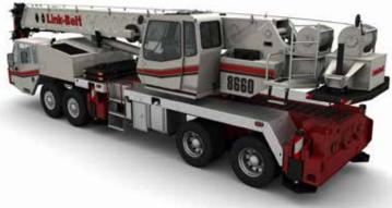
Lightweight **nylon head sheaves** reduce weight and increase capacity.
