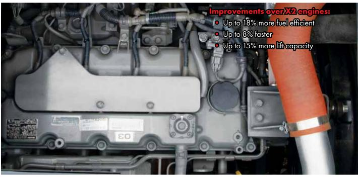
The 80 X3 Spin Ace is powered by a quiet, EPA-certified Final Tier 4 Isuzu engine that strikes the ultimate balance between power, productivity and fuel efficiency...without the need for a Diesel Particulate Filter (DPF)
