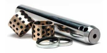
EMS (Extended Maintenance System) chrome pins and grease impregnated brass bushings with graphite inserts reduce wear-andtear and can be found throughout the attachment. This design makes it possible to extend lube intervals to 6 months or 1,000 hours at all pivot points excluding the bucket which is monthly or 250 hours, whichever comes first.
